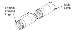
Figure 8 - Vent Pipe Connections
